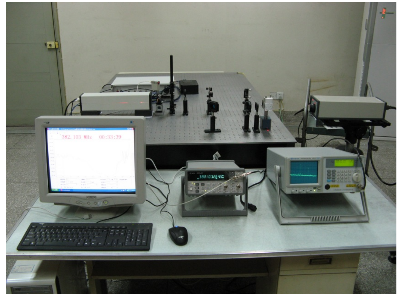
产品与碘饱和吸收基准激光器拍频校准 Products beat frequency calibration with iodine saturated absorption benchmark laser
